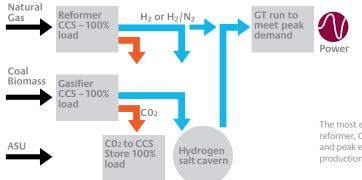
The most expensive assets (gasifier, reformer, CCS) all 'sweat' at 100% load and peak efficiency, even though power production varies.
