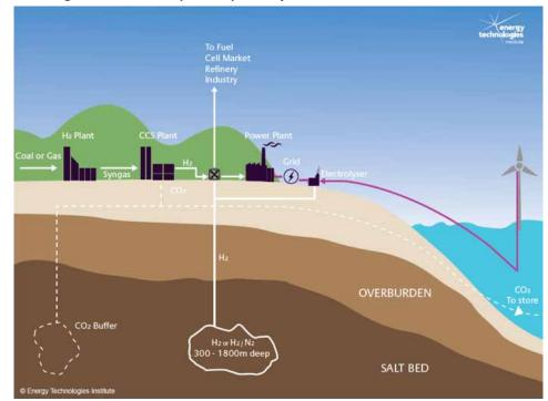
Optional CO<sub>2</sub> buffer storage is shown, to levelise any changes in CO<sub>2</sub> supply to the store caused by other users.
