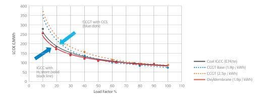
CCGT with CCS is compared to an IGCC with a  $H_2$  store. 'Oxymembrane' means  $H_2$  from methane by precombustion, with separation assisted by membrane (Cachet as noted above).
